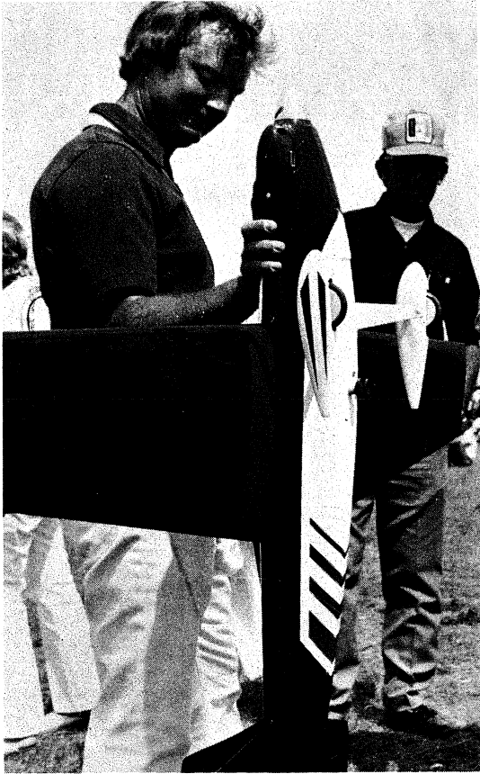
Bob Violett displays Cosmic Wind with super-thin fuselage, minimal frontal area.
