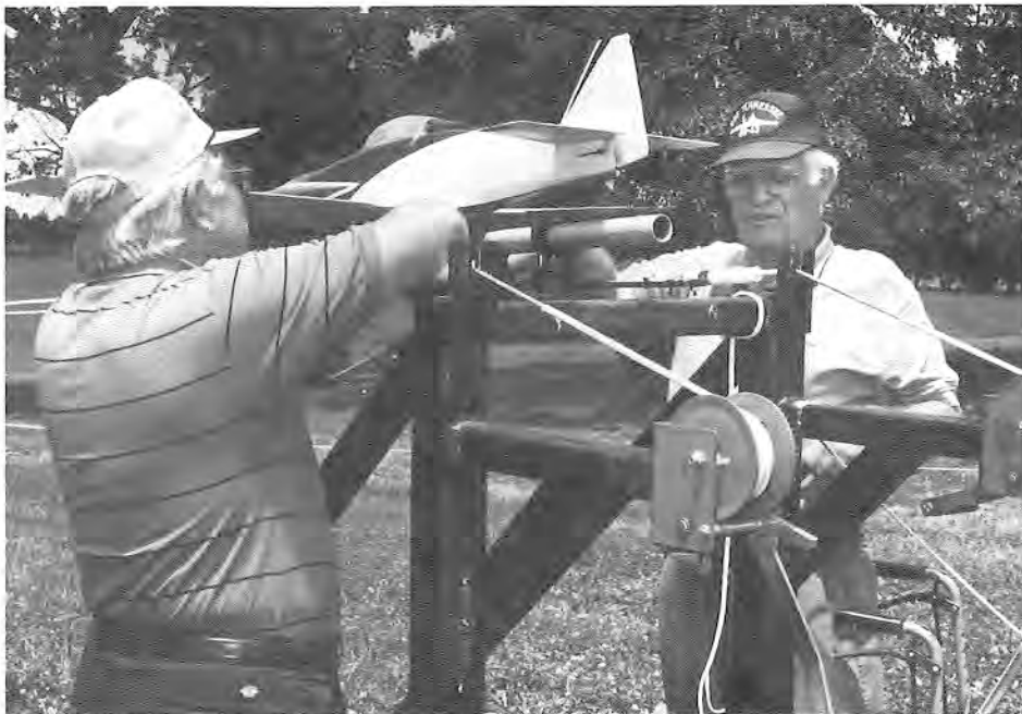
NMPRA's Al Watson and Lee Webster, Tesco Engineering, prepare to launch Formula 1 airplane. The tube under the tail is a solid propellant rocket motor.
