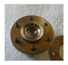
next I removed the crank. In the discussion about after run oil, this is the look of a well saturated motor.
