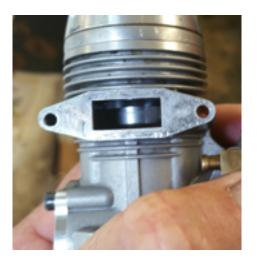
It's setup at no liner shim, 17 under the head. The dry fit is 230 down
