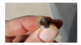
I put in a brand new plug and launched at about 23,500rpm. Another great flight. Much less oil on the bottom of the plane and it was cleaner. Plug had almost no color at all....
