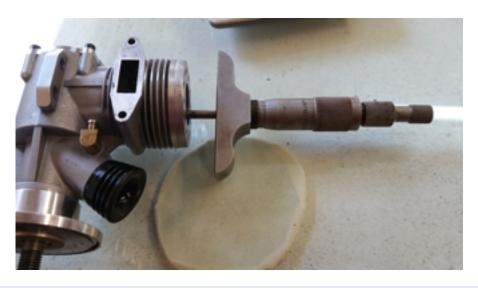
To match the exhaust timing of 197 on the motor a few post before this is not possible, we can't go down only up. I would need to add a .003. To the 197 motor to get it to 198. This would mean one motor is at 189 and one at 191 to get them the same. Last edited by rocket on Sat Dec 10, 2016 3:37 pm, edited 1 time in total.
