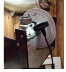
Then its just a matter of spinning the wheel around till the light once again just disappears. Here is what it looks like with no shims under the sleeve. 195.5 -- 196
