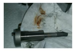
This crank has been in there for a month, after run must not make it this far north so I'm trying a little something with o-ring silicone. Well see after the next disassembly if it helps keep raw fuel from causing rust
