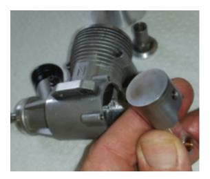
finished the top of the piston with 2000 on the glass top. Here you can see the damage to the inside of the case, it still has the original bearing mike couldn't get out.
