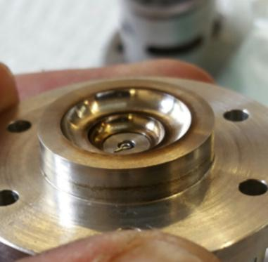
You can see in the next two pics of a gorgilla gripped glow plug install & deformed bowl
