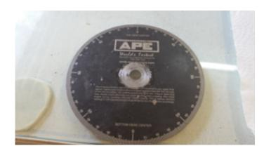
You can tell this wheel has been in use especially for FAI. Buy one with the small hole, I think it's 1/4 inch but I'm prolly wrong. Either way, this one is 5/8 hole. It fits the 15mm FAI stuff better. Just tap the small hole to fit the 5/16 crank. Affix the wheel using a prop and prop nut. Finger tight is ok. Using a head bolt, a nut that the head bolt goes through wrap a piece of wire around the bolt and tighten down.
