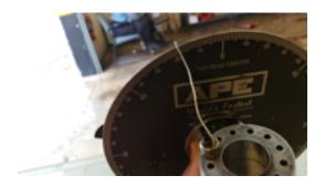
The same setup with no liner shims it's exhaust timing is 198. That's .003 different from the motor before which was 197. The BDC measurement was 980, less the stroke of 791 gives a TDC of 189.
