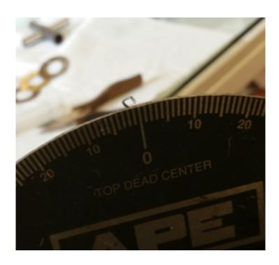
Once your convinced the light is gone, the wire is at 0, rotate the crank the opposite direction NOT UP but down the way around until the light gap disappears again. Look at the indicator, this is your degrees of exhaust timing
