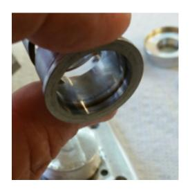
Using Mothers Mag & Aluminum polish, clean up the piston sides and top. Not polishing it to a mirror but just cleaning up the carbon.
