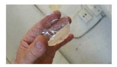
This is penetrating oil and Riches brew, NMPRA 15% it's thinner than lubricating oil. Even after agitation it seperated. Do your own test with your favorite after run to see if it mixes. If you're so inclined to use penetrating oil to prevent rust, do the motor a favor and lube the cylinder and piston with castor befor you flip it over or even worse try to start it.
