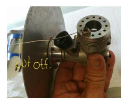
now, looking at the exhaust port on an angel like the pic move the piston until that little light gap disappears.
