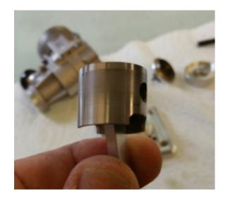
With the liner cut a piece of 1500 or 2000 grit wet dry sandpaper. Using a finger inside the liner roll it back and forth on a flat corner of a tabletop or in this case a glass countertop. All the while moving the Sandpaper in and out, applying light pressure form a crosshatch.
