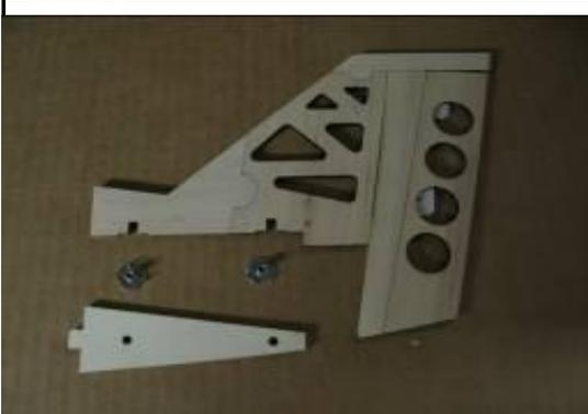
The Fin is assembled as shown. The F-24 light ply plate is used as a clamping platform when the removable tail is used. 6-32 blind nuts are CA'd in place onto F-24 with the "brim" down and the legs up. The tines can be removed to insure proper fit.
