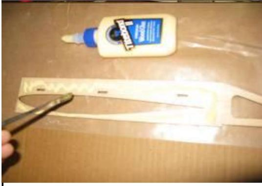
I normally use wood glue for all gluing operations. If you feel more comfortable with CA. Feel free to use it. I use it in spots to act as a clamp to hold parts while drying.
