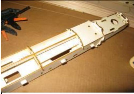
Install F-5 on top of F-4 (in the orientation shown, actually F-5 is to the bottom of the fuselage or the plate that the landing gear attaches to). After you are satisfied with the landing gear plate installation. Glue everything together. Then install F-18 and F-23.
