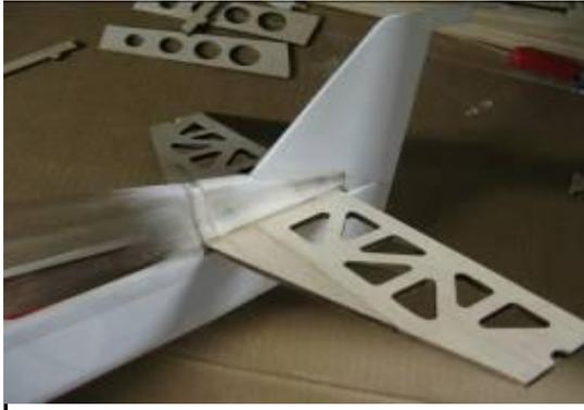
Cover the fin prior to installation. With the stab in place secure F-24 to the fuselage using 6-32 x 1/2" screws. Next install your fin. Remove everything and place a pc of wax paper between the stab and fin assembly then glue the rear fillet in place.
