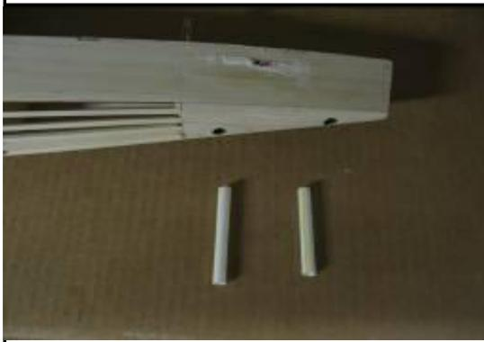
Soda straw (large OD) can be installed to make guide tubes for the tail mounting system.
