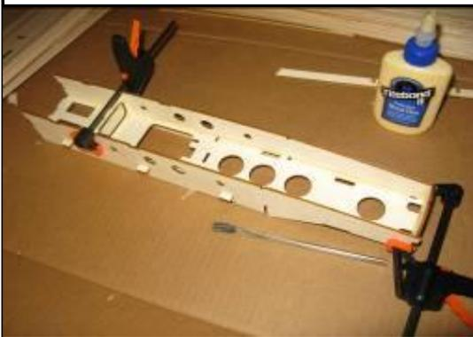
I suggest trial fitting all the pieces together before gluing to understand their placement and order of operations. Use the following series of pictures to aid you through the assembly process.
