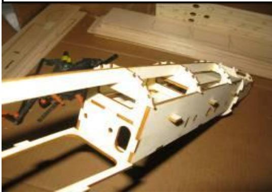
Install F-19. Note the orientation of the ovals. Line up the oval in F-19 to the same side as the oval in front of the servo tray.
