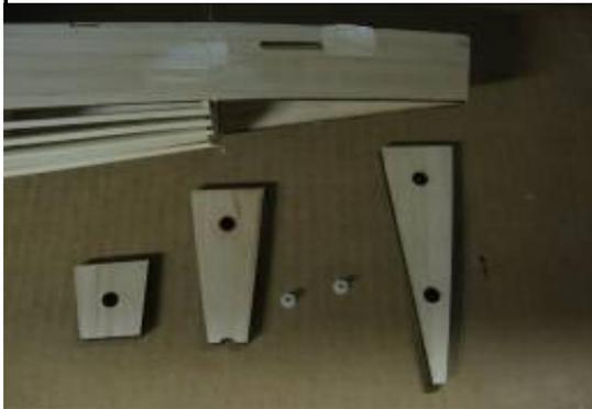
The small nylon shoulder washers shown are installed from the bottom up into F-1 and used as washers when the removable tail is used. The three balsa blocks shown make up the rear bottom of the fuselage (F-26, F-25 & F-27). Prior to installation you should take note of what type of tail skid will be used and make accomdations prior to installation.
