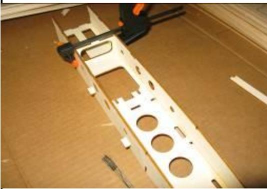
Start with F-10 (inside firewall), F-6 the fuselage light ply doublers, F-3 the servo tray/ battery tray platform and F-17. This can be glued together at this point and clamped til dry.
