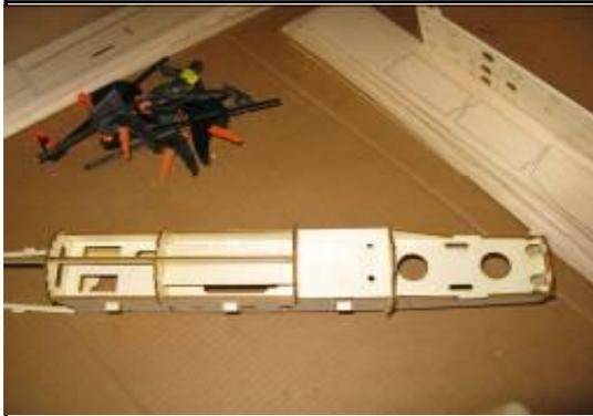
Install the second F-18 bulkhead at the rear of the doubler structure and attach to the F-23 Keel support.
