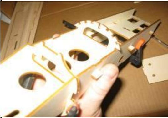
Install F-16 slide into place from the bottom. Hold off on gluing until all of the landing gear plates are installed and glue everything at once. Care should be taken when this former is installed so that F-1 lines up when installed.
