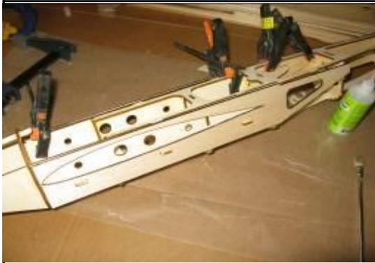
Install both F-7 balsa doublers to the light ply structure. Let this dry before installing the balsa sides.
