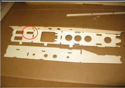
Assembly of the internal light ply structure. Note the position of the servo cut out and the oval just in front of them. This determines the bulkhead orientation as the rest of the fuselage is completed.
