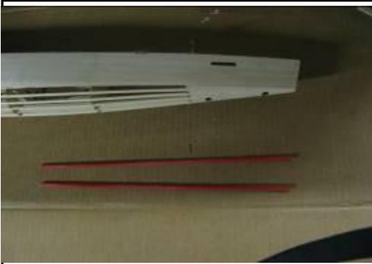
I have been using the RED outer sleeve for pushrod guides and solid 2-56 rods for pushrods without the white or yellow sleeving. Note, because the Fin assembly is only 3/16" wide and the rear of the fuselage is 1/4" wide you may choose to taper rear more to get a better fit.
