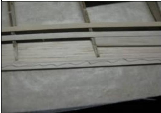
NOTE: the bottom sheeting must be tapered to receive the top trailing edge sheeting. I used a combination of a razor plane and a T-Bar to sand this taper. Also the trailing edge per NMPRA rules cannot be any thinner than 1/16". Therefore, you should end up with the T.E. being the thickness of the upper sheeting.
