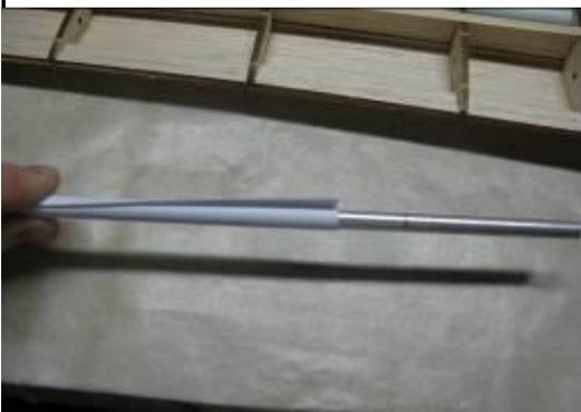
Using a pencil or wooden dowel, roll the paper tightly as shown.
