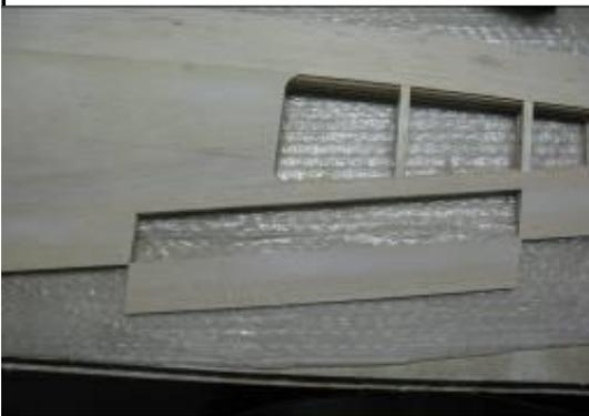
Using the tick marks on the sheeting cut out the aileron as shown. I normally use an X-Acto knife to cut along the hinge line from the top and a Razor saw to cut the ends. I use 4 hinges for attaching this surface.
