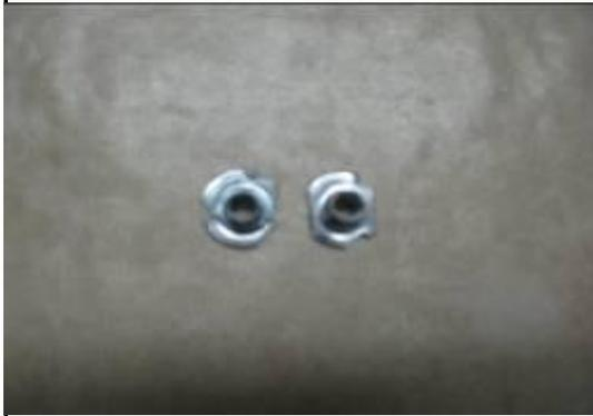
Trim, the 1/4-20 T-Nuts to fit on the inside of the W-2 rib.
