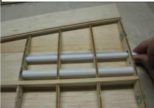
Now slide the whole thing into the wing panel and line up the end of the paper tube with the outside of the W-5 rib. CA in place and trim the outside edge.
