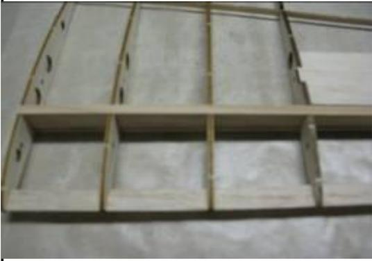
At this point you can remove your panel assembly from the piano wire jigs. Install your top and bottom main spruce spars (1/4" x 1/8" not supplied).
