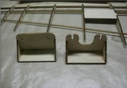
Assemble the three wing assembly jigs as shown. They are built from 4 pcs, (2 gussets, a floor and a vertical support). These will be used along with 2 pcs of 1/8" piano wire not supplied. The end jigs should be clamped or screwed to your surface and should be square to one another. The ribs will be pushed up against these supports during the assembly process. And it is important that they remain square during the initial stages of assembly.
