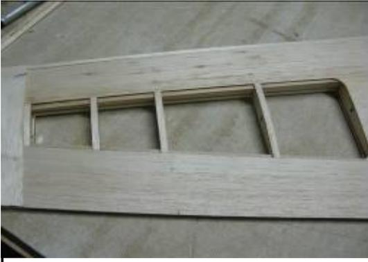
Install the 1/16" x 1/4" balsa cap strips (Not supplied) to the top and bottom of the wing.
