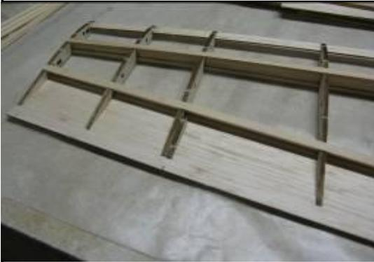
Install W-19 (two per panel, aileron end support) to the inside of both the W-8 and W-5 ribs. (the one in the picture is at the W-8 rib).
