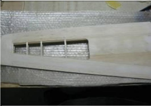
Final sand and shape the wing. Fill as necessary.
