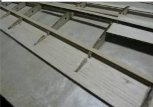
Next, lay one W-18 (aileron hinge line support) across the top of your ribs. Line up the leading edge of W-18 with the leading edge of the W-19 aileron support wedges. Mark the W-6 and W-7 ribs as they will be cut to allow W-18 to sit flush on the bottom sheeting.
