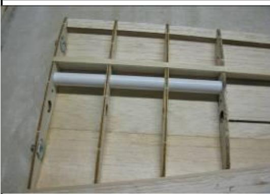
Once the glue has dried, turn the wing over and install the cardboard joiner tube. This can be secured in place using CA on the outside. (NOTE: this is the hole closest to the leading edge. This tube is needed for the other panel and for the fuselage. Therefore be careful with the trimming of the tube.
