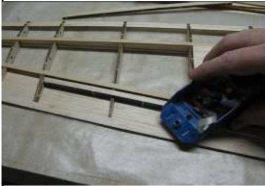
Using a razor plane, trim the balsa support blocks just installed to match the contour of the wing.
