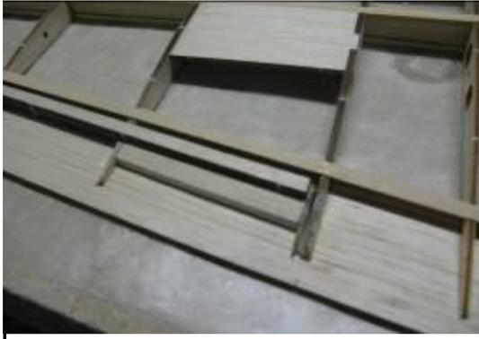
Install the second W-18 component on top of the first. At this time you can install aileron control horn support (un-numbered but located on the 3/16" balsa sheet where the W-18's were removed).
