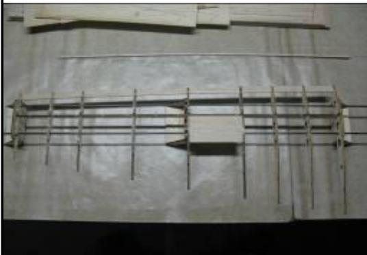
Slide your wings onto the 1/8" piano wire. NOTE makes sure before assembling the second panel you are building a left and right wing. Then install your leading edge alignment component W-12. lastly, install your balsa servo floor between W-5 and W-6. (THIS PIECE DOES HAVE A SPECIFIC ORIENTATION. THE FRONT EDGE SHOULD BE FLUSH WITH THE MAIN SPAR.)
