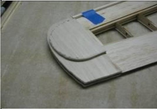
Using the supplied 1/8" wing tip as the foundation for the wing tip. Build up the tip using scrap balsa and glue the tip in place.
