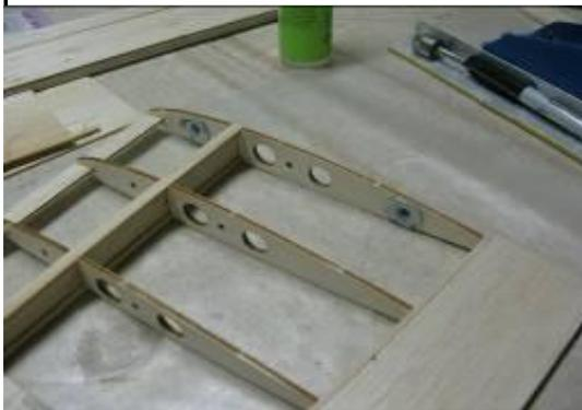
Install the trimmed 1/4-20 T-Nuts. Note: you may need to slightly countersink or bevel the inside edge to get the nuts to sit flush. CA or Epoxy in place.
