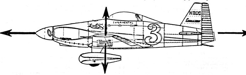
In the above diagram, the vectors of the four major forces acting on an aircraft in unaccelerated level flight are shown. Lift equals Weight and Thrust equals Drag. Thrust is all the force that your engine and prop can produce when the aircraft is at top speed. If you can't get any more thrust from your engine or prop, then you have got to reduce drag to go faster.
