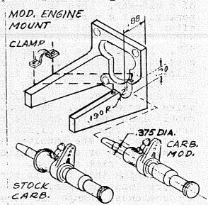
The center of the groove is cut .887 from the back of the mount. You then drill and tap two 4-40 holes on each side of the groove. Then cut a small strap and drill two holes in a small metal strap to clamp the unit in the mount. Then run Hot Stuff around the needle valve unit and screws to cement the whole mess in the mount. Cut a hole in the top or bottom of the fuselage for the needle valve exit and install the mount and needle valve unit.
