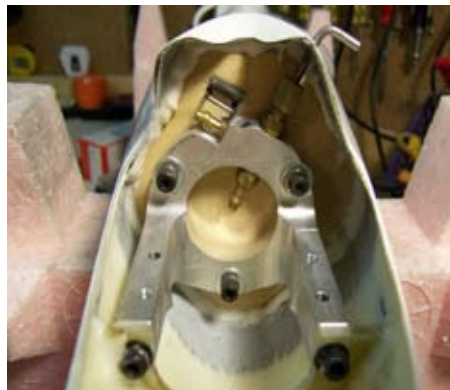
Photo #1: Motor mount installed in Sweet-V fuselage. Note fuel shutoff wire loop and carbon rod shown just above the top of the mount
