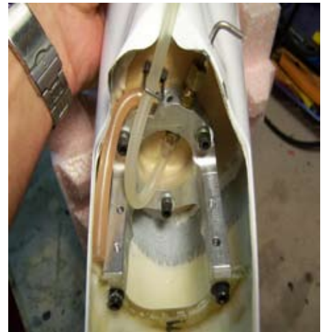
Photo #2: Fuel lines installed. White line is fuel supply line coming from the fuel tank, over the piece of carbon rod and through the wire loop
