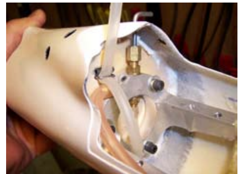
Photo #3: Wire loop pulls the white fuel tubing into the "valley" created between the carbon rod and pink fuel line. Shutoff is achieved.
