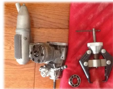
A well run Thunder Tiger Pro 40, with at least 65 heats on it since it was last maintained. Note stock muffler and Battery Post puller used to remove the thrust washer.
