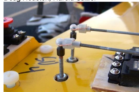
Safety wire connection on aileron torque rods. Refer to District 3 column for description.
