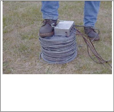
This system is light weight, simple & easy. The sheathed cable is less than  $\frac{1}{4}$  inch in diameter and the 350 feet of wire will roll onto a spool that is about 18 inches in diameter. Because the system is relay operated with the battery next to the relays, there are no line losses and the lights are bright. The 350-foot switch lines are just that, there is no time delay.
