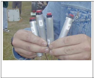
The switches that are used to flash the turn lights are "momentary on switches"; that is, you push and hold the switch to turn on the light. Purchase these switches at an electronic supply house. We used some <sup>3</sup>/<sub>4</sub> inch diameter aluminum tubing about 4 inches long with some machined end pieces to make a nice hand held housing.
