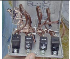
Now do the wiring from the relays to male plugs on the turn lights. Use the female plug end from the 14 gauge extensions cords that were cut to wire the 3 prong light plugs. Solder to pin 85 & 87 of each relay so that you have (1) female plug for each of the turn lights. The diagram above shows the wiring proceedure.
